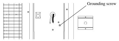
2. Feed a power supply cord (not included) through the access cover and connect it with the two leads. The ground line should be connected to the grounding screw. The two connectors must be insulated. Put the access cover back in place.
